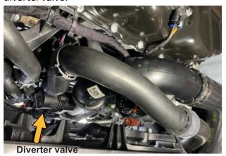
2) Using a T25 Torx driver, remove the 3 screws holding the diverter. NOTE, the tight location makes it difficult to access one of the screws. You can either use a flexible drive extension (or series of extensions, wobble drive/universal joints), or remove the screws that hold the charge pipe to the engine block, then remove the rubber intercooler hose so you can gently pull the charge pipe forward. This gives you better access to the last screw on the diverter valve:
