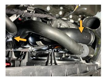
3) Unplug the connector and remove the factory diverter valve:
